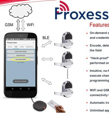
The Proxess Sync™ mobile phone app synchronizes changes from the AxessIQ™ software to the LoxIQ™ locksets and it uploads the Audit Trails from the locksets to the software. You can also encode cards for users that have been added in the software. The app can be issued to an unlimited number of phones and users and connected with an unlimited number of doors.
