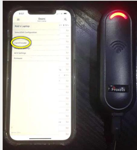
Tap "Card Encoder" and make sure the Enrollment Reader (ENR) is within 12" for the initial connection. The screen will state that it is looking for the ENR. Once connected, the ENR can be up to 20' away.
