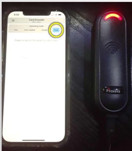
To Wipe & Delete a credential, Click on the "Wipe" button. Then place a card onto the reader surface. The blue LED shows the card is being read and/or written to.
