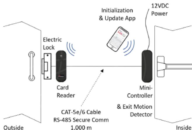
The *Proxess Mini-IQ* is the simplest and most cost-effective door controller to install and operate, and rounds out the Proxess product line, supporting applications at every door type;
