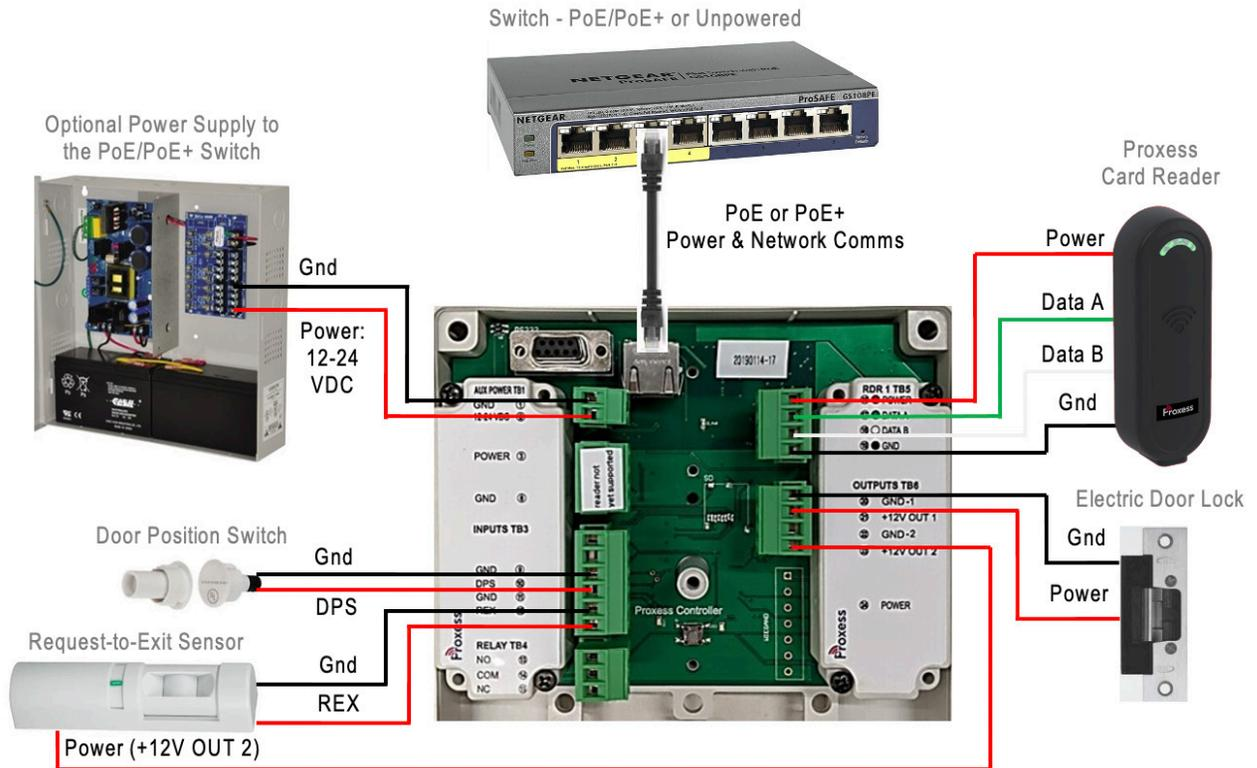
**POWER NOTE:** Verify the voltage and current requirements of your selected electric door lock prior to connecting to the Proxess BoxIQ. If you have any questions on the suitability of a direct power connection from the BoxIQ, please select and use a separate power supply and connect per the above drawing.
