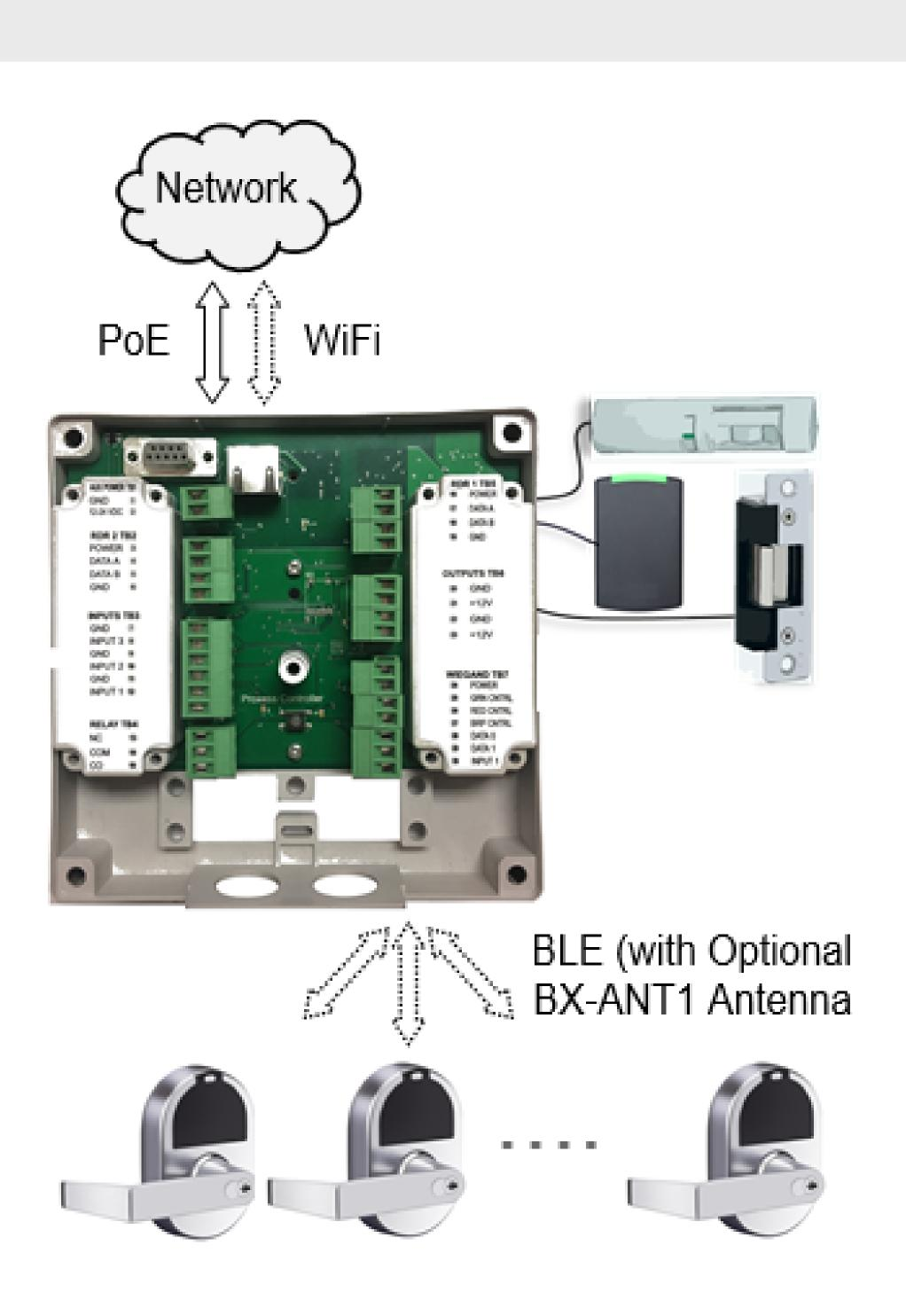
The BoxIQ™ is the Proxess solution for the more conventional access control doors using a reader. The BoxIQ™ wirelessly communicates with your Proxess electronic locksets "On-Demand" (with the separately ordered BX-ANT1 antenna). The BoxIQ™ also allows the user to control commands and further monitor access to high-security portals using the ProxessIQ™ software.
