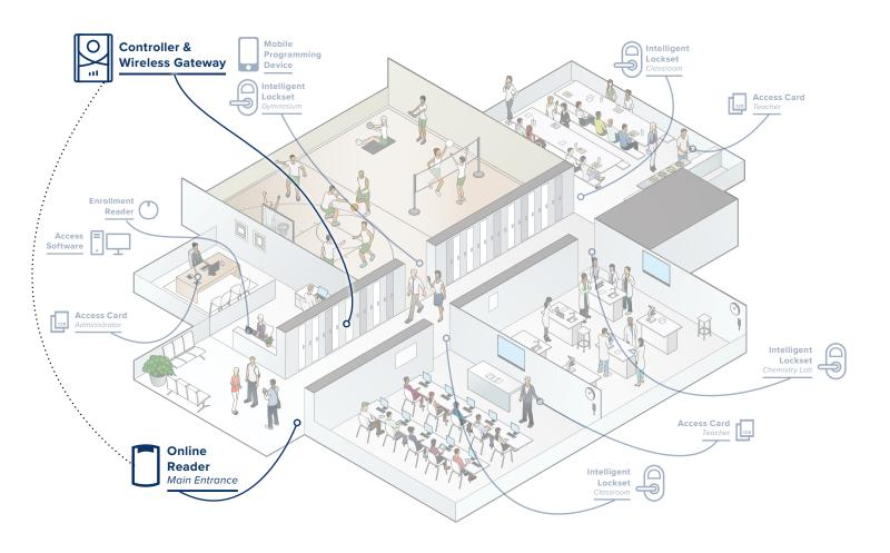
BoxIQ™ door controllers control 2 doors and connect to the customer's network with a PoE or PoE+ cable, or WiFi. These **online** doors download transactions off the cards from the locksets they visited. These doors upload changes made in the software, onto the card, for the **offline** locksets they will visit. Cards can be set to auto-expire each night. Entering an **online** door re-validates the card for all the **offline** locksets visited that day.
