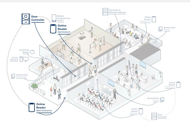
BoxIQ<sup>™</sup> door controllers control 2 doors and connect to the customer's network with a PoE or PoE+ cable, or WiFi. These doors are always online. The card readers are connected via 2-wire RS-485, using bi-directional communication, for greater security and integration.
