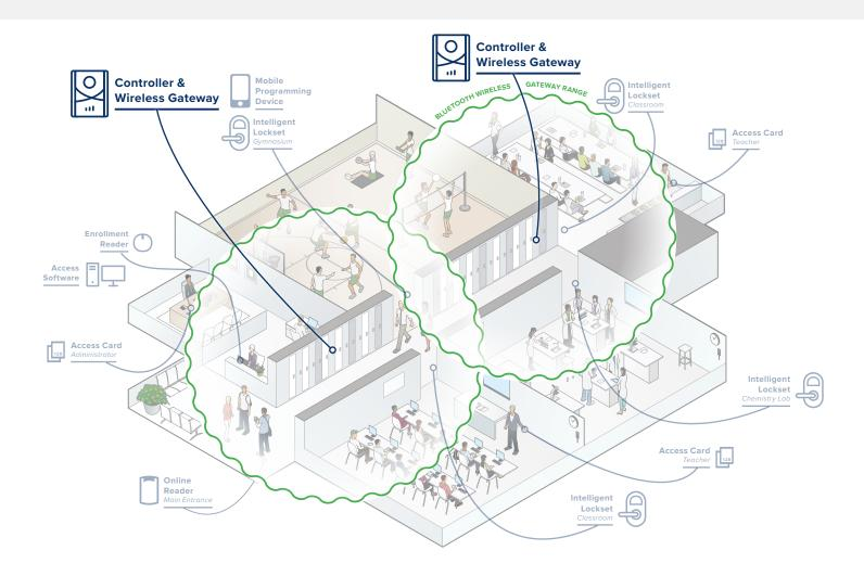
BoxIQ™ is also a Bluetooth Gateway & connects to the customer's network with a PoE or PoE+ cable, or using their WiFi network. Add Gateways anywhere on the property, where on-demand performance is desired for specific locksets. They communicate to the locksets via BLE (Bluetooth Low Energy). Each LoxIQ™ is registered to a gateway.
