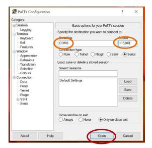
2. A black screen will appear during the opening process and the Putty programming tool will then open. The top of the window confirms your computer's comm port and the body of the screen shows the version of the BoxIQ, any IP address it may have, its unique identifying Fingerprint, any ACS (access control system) it may be connected with and if it has been linked and trusted with an ACS.
