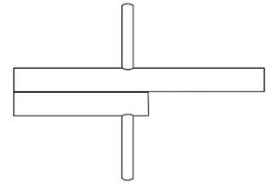
Cylinder and Core Testing Wrench
