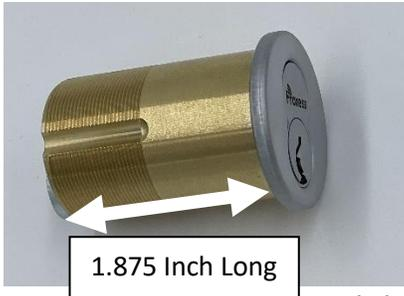
Due to the extra thick trim that houses RF and battery components, Proxess mortise locks require special length (1 <sup>7</sup>/<sub>8</sub> inch) cylinders (similar to Schlage style cam). When using other manufacturers' cylinders, ensure that you have the proper 1 <sup>7</sup>/<sub>8</sub> inch long cylinder.
