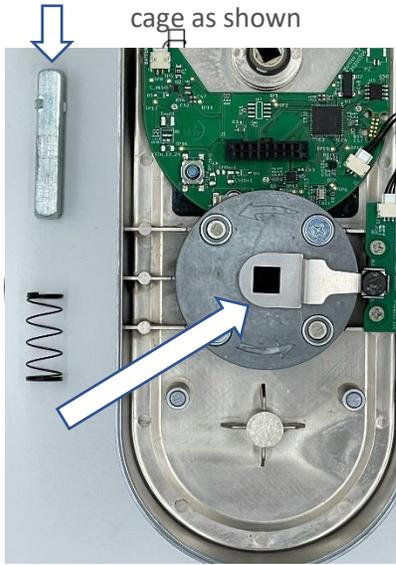
**Note:** The spring is not attached to anything and can be easily misplaced. Use caution when installing the spring.
