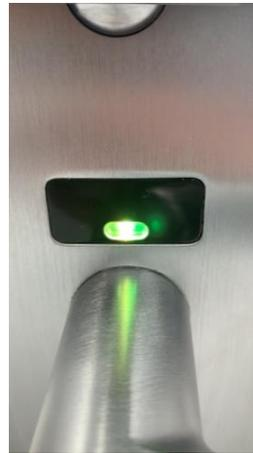
The interior light will illuminate in colors, and you will hear a beep, indication that the power is on. Turn the lever and make sure the lever is free to rotate.
