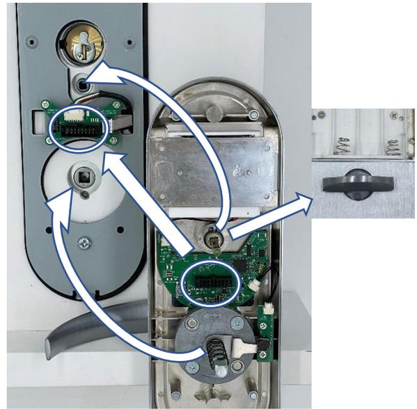
Align the spindles and EZ connect with the chassis and place it onto the interior backplate.
