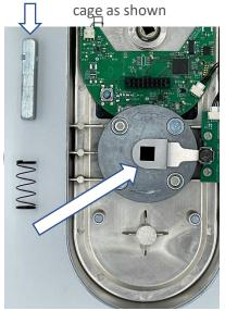
**Note:** The spring is not attached to anything and can be easily misplaced. Use caution when installing the spring.
