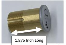
Due to the extra thick trim that houses RF and battery components, Proxess mortise locks require special length (1  $^{7}/_{8}$  inch) cylinders (similar to Schlage style cam). When using other manufacturers' cylinders, ensure that you have the proper 1  $^{7}/_{8}$  inch long cylinder.
