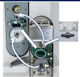
Align the spindles and EZ connect with the chassis and place it onto the interior backplate.
